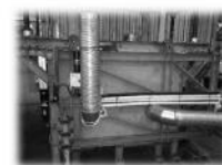
Die preheater Arconic internal design
